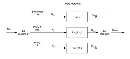
Figure 22: E-DCH hybrid ARQ functionality
